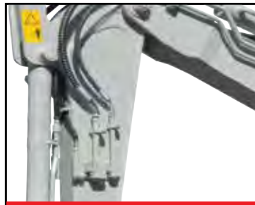
1st, 2nd, 3rd Auxiliary Lines
