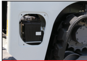
Battery Access Panel
