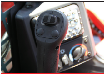
Pilot Operated Controls
