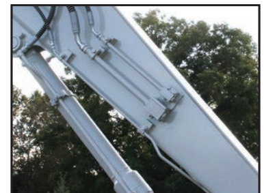
Auxiliary Hydraulic Lines
